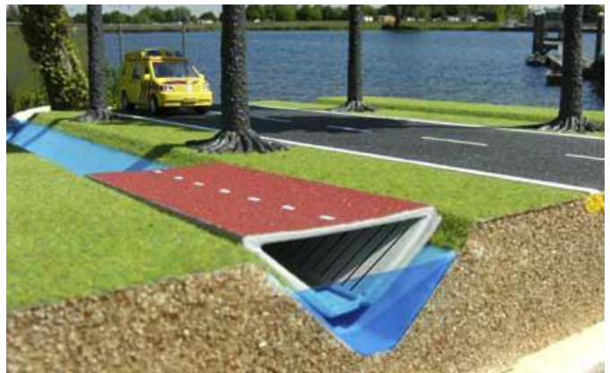
Combination of drainage and cycle path
